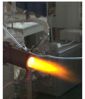
Water vapour plasma torch for the organic waste treatment
