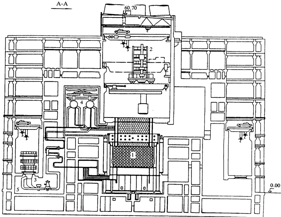
**Fig. 1.5** Cross-section A-A of one unit of the Ignalina NPP [2]
