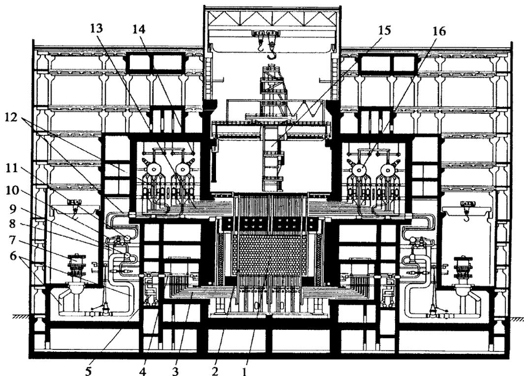
**Fig. 4.1 General view of the reactor**
