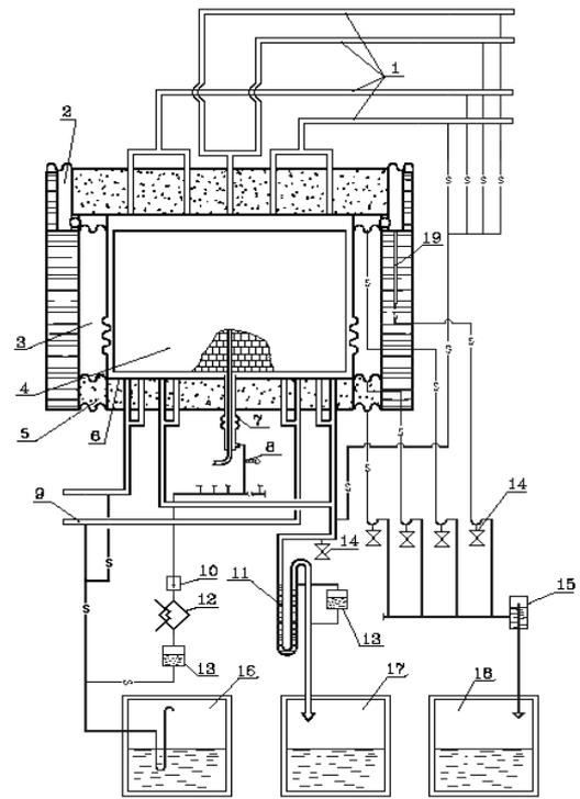
**Fig. 4.19 Block diagram of the reactor draining system**
