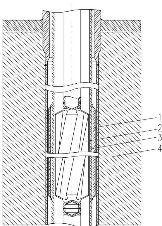
**Fig. 4.7 Fuel channel shielding plug**
