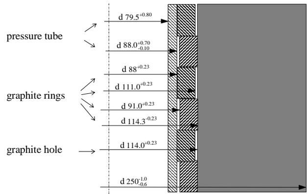
**Fig. 4.11 Graphite and zirconium interaction zone**
