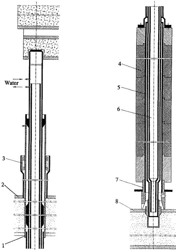
**Fig. 4.15 Reflector - cooling channel**
