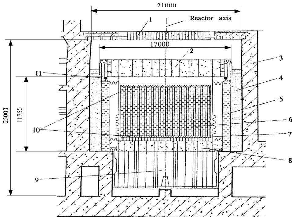
**Fig. 4.4 Cross-section of the reactor vault**
