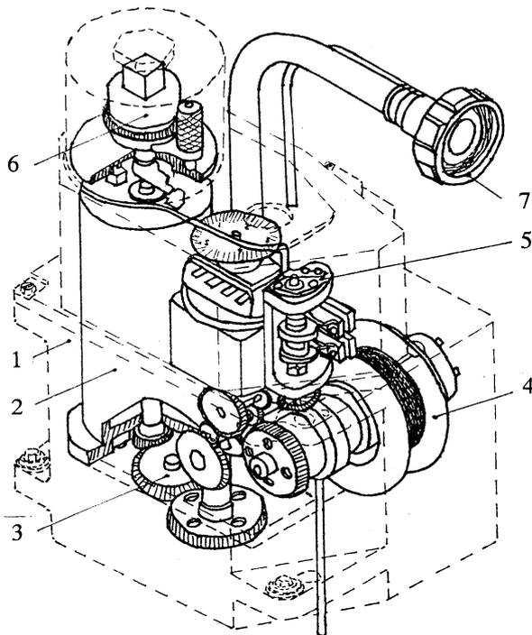
**Fig. 4.18 Control rod drive**
