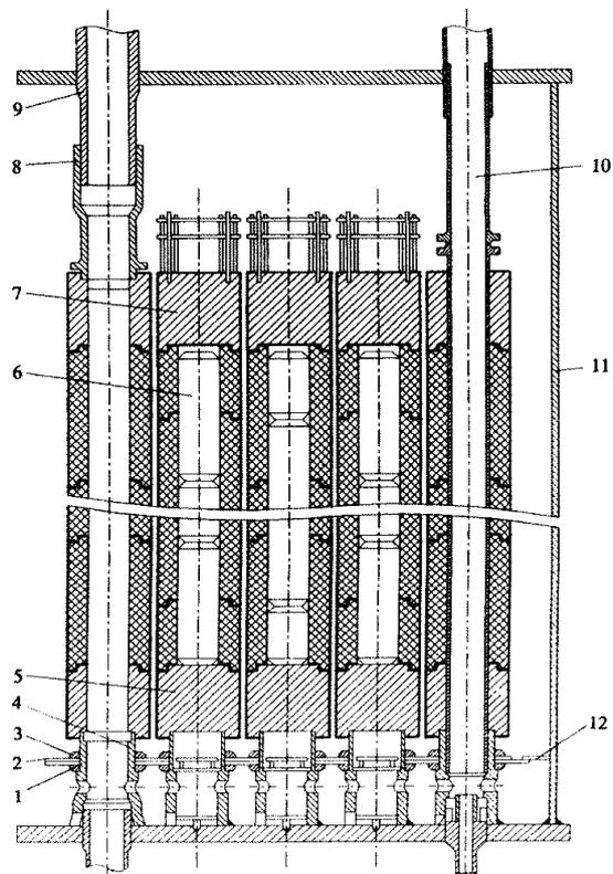
**Fig. 4.3 Segment of the graphite stack**
