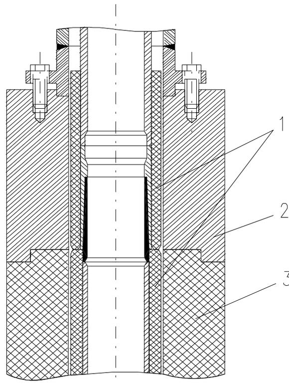
**Fig. 4.8 Shielding sleeves in the top reflector**
