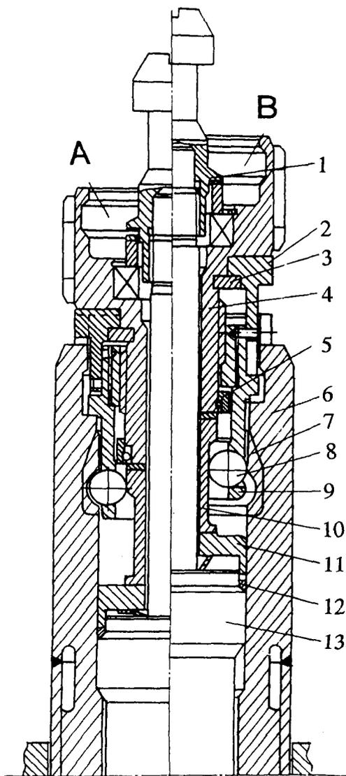
**Fig. 4.12 Fuel channel seal plug (for unit 1)**
