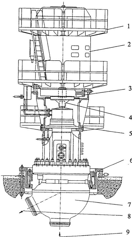
**Fig. 5.9 The pump equipment of the RBMK type reactor**
