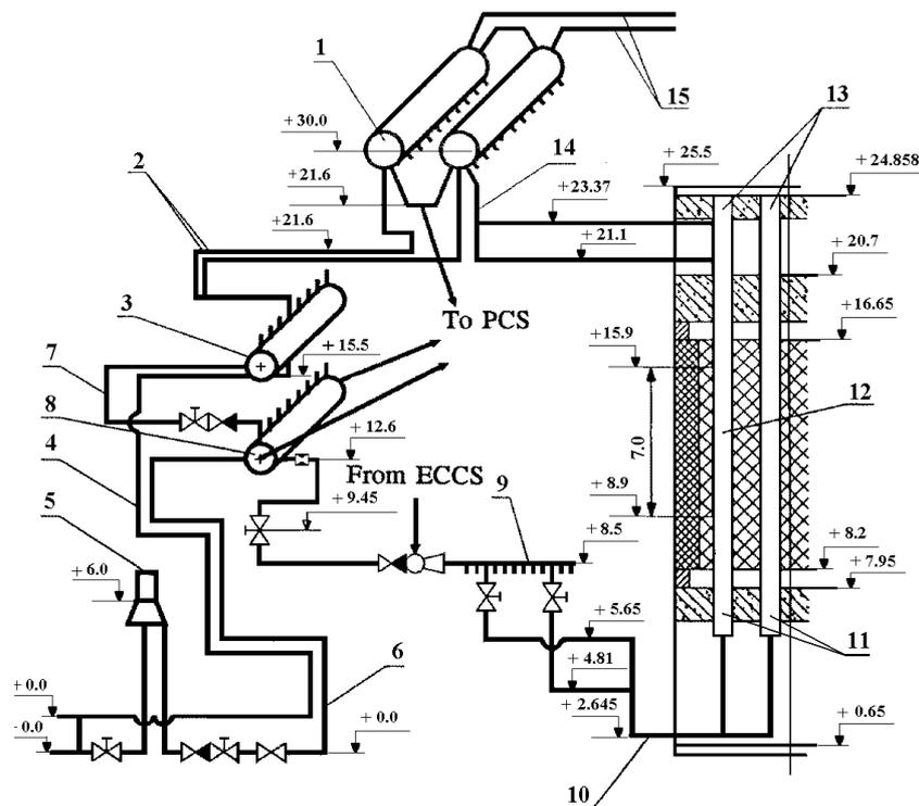
**Fig. 5.2 Elevations of the MCC**
