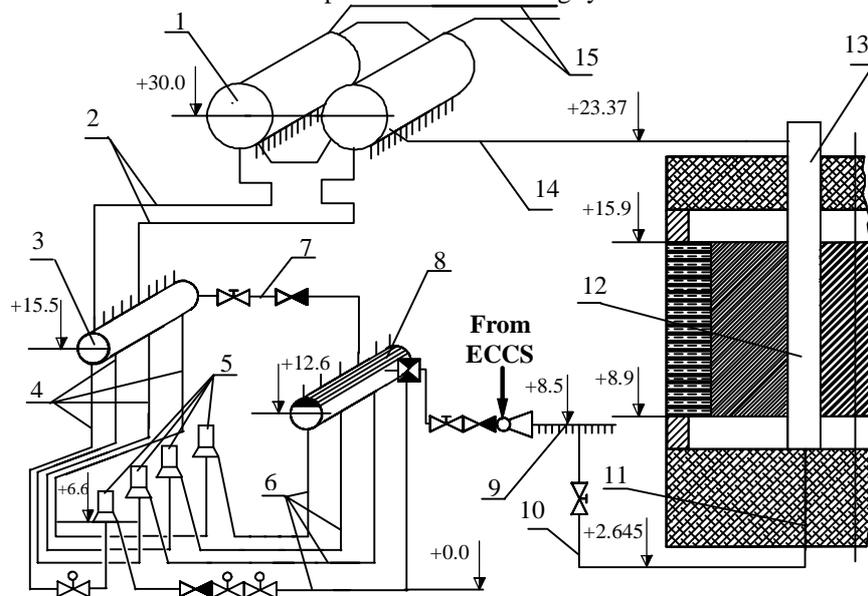
**Fig. 5.1 Schematic representation of one loop of the main forced circulation circuit**
