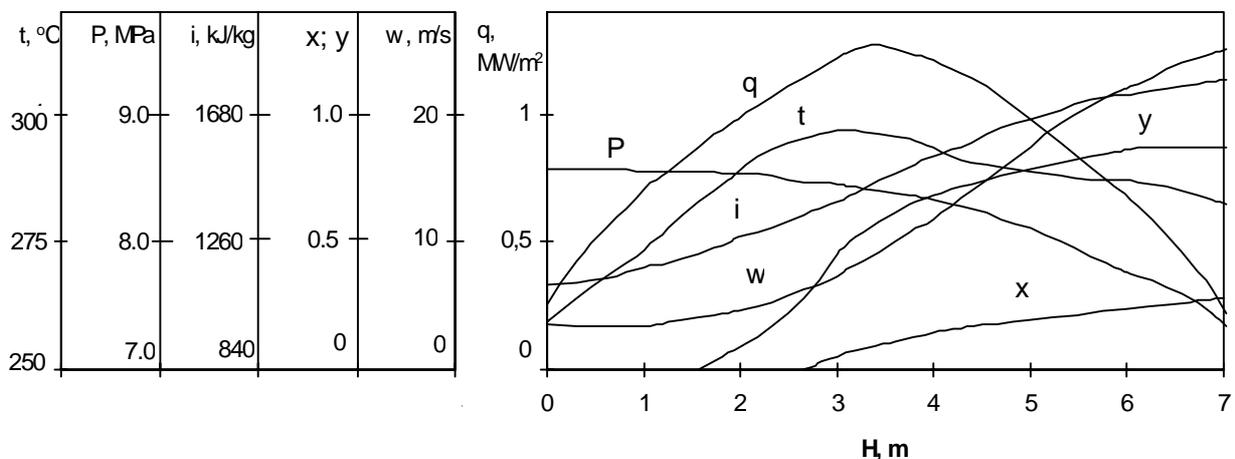
**Fig. 5.6 Vertical variation of coolant parameters along the maximum designed power 4.5 MW fuel channel [35]**
