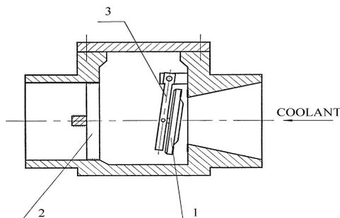
Fig. 5.12 A schematic representation of the GDH check valve
