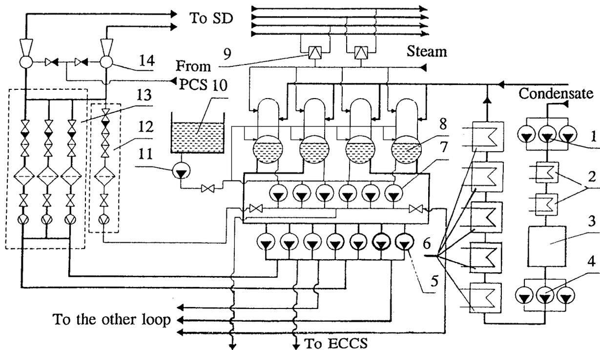
**Fig. 5.14 Water feedback system**
