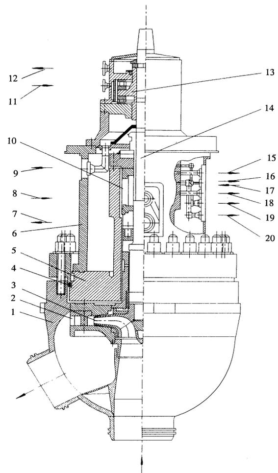
**Fig. 5.10 Schematic of the RBMK-1500 pump**
