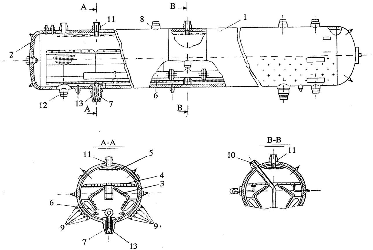
**Fig. 5.7 Separator drum**
