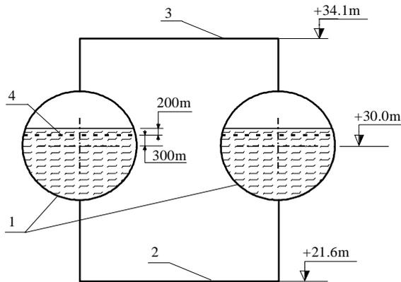
**Fig. 5.8 Connections at the liquid and steam level between separator drums**
