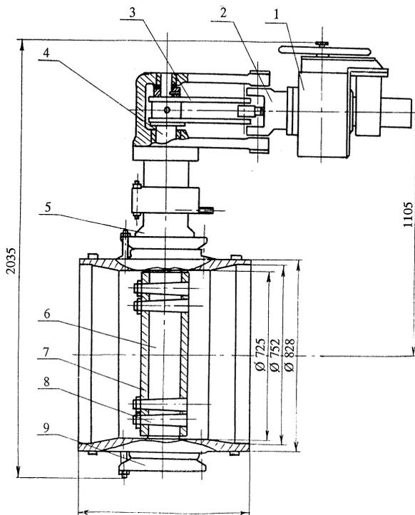
**Fig. 5.11 A schematic representation of the throttling-regulating valve**
