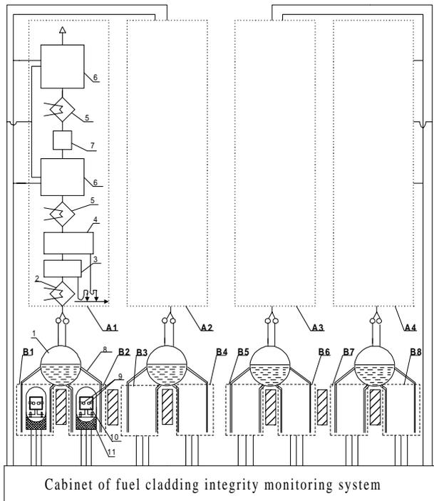
**Fig. 5.17 Schematic of fuel cladding integrity monitoring system**
