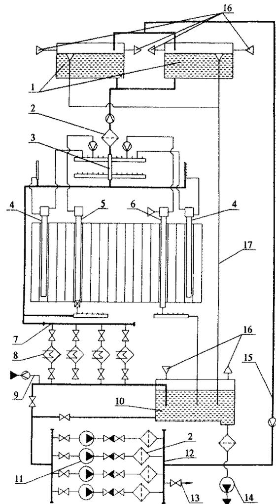
**Fig. 5.16 Control rod cooling circuit**
