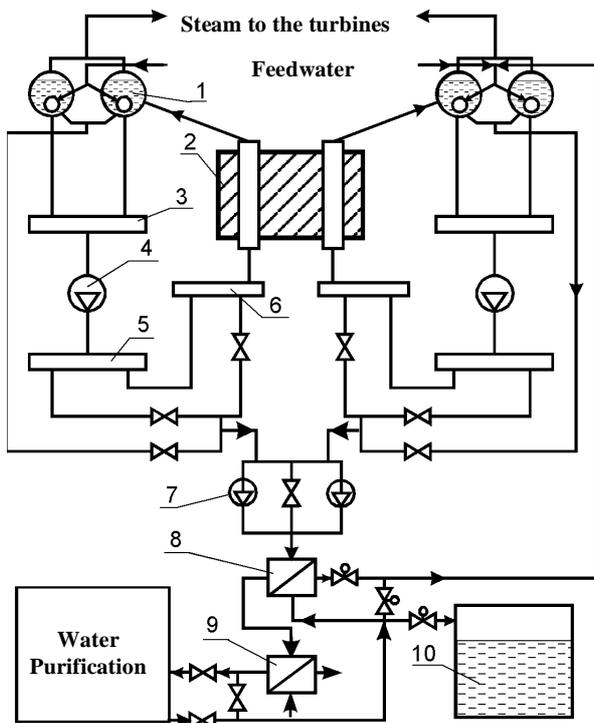
**Fig. 5.15 A schematic representation of purification and cooling system**
