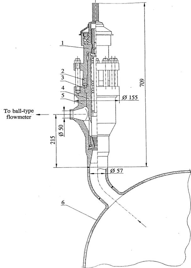
**Fig. 5.4 Isolation and control valve**
