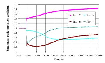
Figure 10 Spearman's rank correlation coefficients for suspended aerosol mass (only the parameters with coefficient exceeding 0.3 at least at one point are highlighted)
