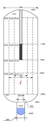
Figure 3 Nodalisation scheme of PHEBUS containment
