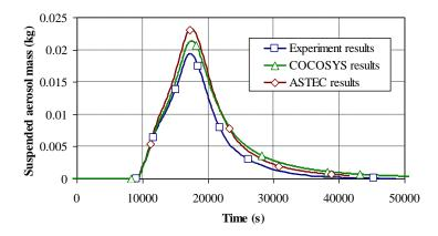
Figure 12 Aerosol mass suspended in the containment atmosphere
