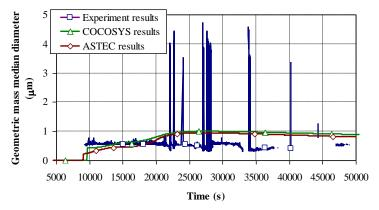
Figure 13 Aerosols geometric mass median diameter in containment atmosphere
