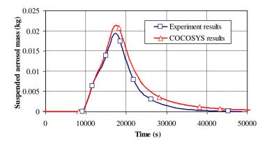
Figure 6 Suspended aerosol mass in containment
