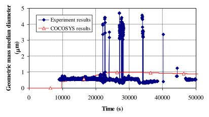
Figure 8 Aerosol geometric mass median diameter
