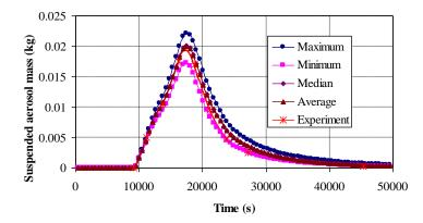
Figure 9 Suspended aerosol mass (maximum, minimum, median, average and experiment values) in containment
