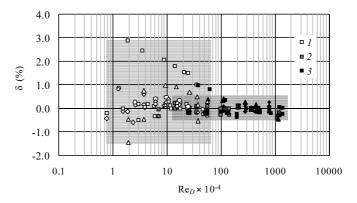
Fig. 7. Comparison of experimental results obtained using meters of various types and sizes under atmospheric and increased pressures:  $1 - \nu = 15.4 \cdot 10^{-6} \text{ m}^2/\text{s}$ ;  $2 - \nu = 2.74 \cdot 10^{-6} \text{ m}^2/\text{s}$ ;  $3 - \nu = 0.44 \cdot 10^{-6} \text{ m}^2/\text{s}$
