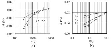
Fig. 17. Density measurement errors under changing pressure: a) measuring silicone oil No. 2 (I - 0.1 MPa; 2 - 0.65 MPa; 3 - 15 bar); measuring water (I - 0.1 MPa; 2 - 0.65 MPa)
