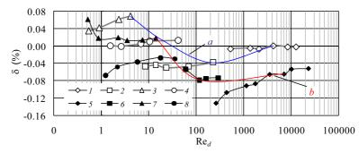
**Fig. 13.** Errors of two types of MM considering Re<sub>d</sub> in flows of various liquids: 1, 2, 3 and 4 – "U" type; 5, 6, 7 and 8 " $\Omega$ " type; 1 and 5 – water; 2 and 6 – oil No. 1 (v = 60  $\cdot 10^{-6}$ , m<sup>2</sup>/s); 3 and 7 – oil No. 2 (v = 600  $\cdot 10^{-6}$ , m<sup>2</sup>/s); 4 and 8 – oil No. 4 (v = 200  $\cdot 10^{-6}$ , m<sup>2</sup>/s). Curves a and b were drawn through the points of one flow rate  $Q = 5.5 \cdot 10^{-5}$  m<sup>3</sup>/s of both meters
