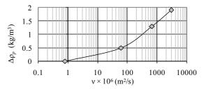
Fig. 12. MM density error dependence on liquid viscosity
