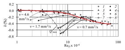
Fig. 9. RM errors when the measured liquid is: 1 and 2– diesel fuel in laboratories and correspondingly operating places, 3 and 4 – kerosene Jet-A1 in laboratories and operating places, 5 and 6 – A-95 petrol in laboratories and operating places, 7 and 8 – DN100 and DN65 flow meters measurements with liquid Exxol D80
