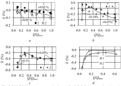
**Fig. 8**. RM (DN 100) errors measuring in: *a* – diesel fuel; *b* –kerosene Jet-A1; *c* –A-95 petrol flow: *I* and *2* – measurements under laboratory and natural conditions, respectively; *d* – the flow of liquid Exxsol D80: *I* and *2* –DN100 and DN65 size meters respectively under laboratory conditions
