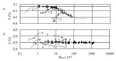
Fig. 11. Comparison of RM and TM errors variance according to Re<sub>D</sub>: *a* RM: *1*, *2* and *3* – respectively  $v = 4.6 \cdot 10^{-6}$ ,  $2.3 \cdot 10^{-6} - 1.7 \cdot 10^{-6}$  and  $0.7 \cdot 10^{-6}$  m<sup>2</sup>/s; *b* TM: *1*, *2* and *3* – respectively  $v = 15 \cdot 10^{-6}$ ,  $2.74 \cdot 10^{-6}$  and  $0.44 \cdot 10^{-6}$  m<sup>2</sup>/s
