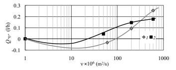
Fig. 15. MM "0" flow rate dependency on the measured liquid viscosity: I -" $\Omega$ " and 2 - "U" type meters
