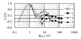
**Fig. 6.** Error dependence of two TM (type C, DN 150) on Re<sub>D</sub>: 1, 3 – atmospheric pressure; 2, 4 – 0.6 MPa pressure
