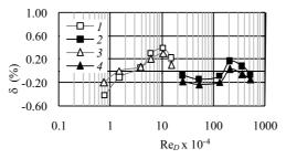
**Fig. 4.** Error dependence of two TM (type A, DN 150) on Re<sub>D</sub>: 1, 3 – atmospheric pressure; 2, 4 – 3.4 MPa pressure
