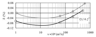
**Fig. 14.**  $1 - "\Omega"$  and 2 - dependency of "U" type MM errors on viscosity of the measured liquid
