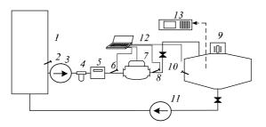
Fig. 1. Equipment scheme for investigation of liquid viscosity influence: 1 – liquid tank; 2, 6, 8 and 10 – temperature meters; 3 – pump; 4 – filter and air (gas) separator; 5 – liquid density and viscosity meter; 7 – the investigated RM; 9 – flowing liquid volume or mass measurement system; 11 – pump returning fluid to the tank; 12 – computerised system for measurement data collection and processing; 13 – liquid density and viscosity meter
