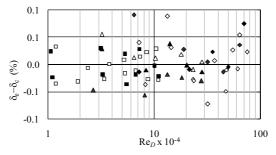
Fig. 10. Difference between the experimental results and data obtained using the numerical model  $(\delta_e - \delta_c)$  for the same viscosity
