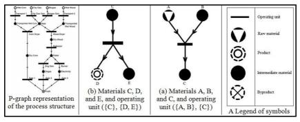
Figure 3. Principle of PNS structure using P-graph method
