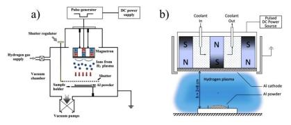
Fig. 2.1. Vacuum system (a) and magnetron (b)
