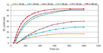
**Fig. 3.13.** Hydrogen production using 0.05 g of Al powder and different volume of water (10 ml, 20 ml, 30 ml, 40 ml, 50 ml and 100 ml)
