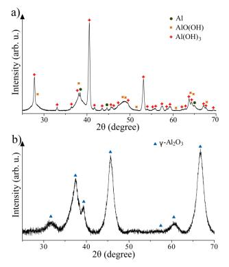
**Fig. 3.17.** XRD results for the by-product obtained after the reaction between the modified aluminium powder and distilled water (a) and the complete transformation of aluminium hydroxide into gamma alumina after heating at 500 °C (b)
