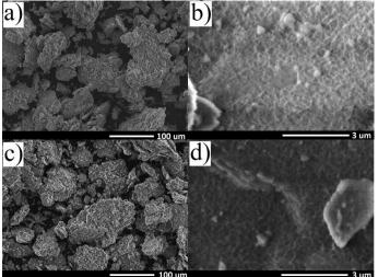
**Fig. 3.16.** SEM images of the initial by-product (mainly Al(OH)<sub>3</sub>) surface obtained after the aluminium/water reaction (a–b) and the gamma alumina surface obtained after the aluminium hydroxide was heated at 500 °C (c–d)
