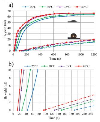
**Fig. 3.11.** Temperature influence on H<sub>2</sub> generation using 0.05 g of modified and unmodified Al powder with 40 ml of water (0.2 g of NaOH dissolved in 100 ml H<sub>2</sub>O) (a) and enlarged view of reaction start (b)
