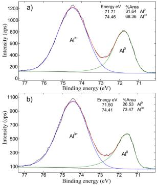
Fig. 3.8. Al2p peak fitting of unmodified (a) and plasma modified (b) Al powder at 250 W, 8 cm for 1 h
