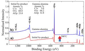
Fig. 3.18. XPS surface elemental composition analysis for the initial by-product obtained after the aluminium/water reaction (a) and the gamma Al<sub>2</sub>O<sub>3</sub> formed after the hightemperature treatment of the reaction by-product at 500 °C (b)
