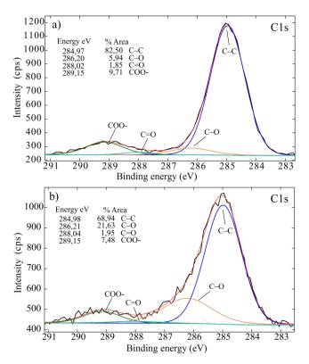
Fig. 3.6. C1s peak fitting of unmodified (a) and plasma modified (b) Al powder at 250 W, 8 cm for 1 h
