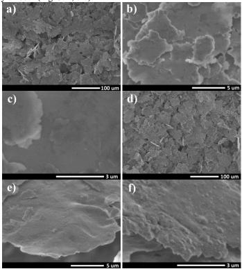
Fig.3.4. SEM images of untreated Al powder (a-c) and  $\rm H_2$  plasma modified at 250 W and 8 cm distance for 1 h (d-f)
