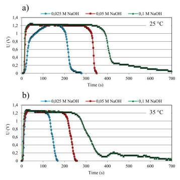
**Fig. 3.15.** Electricity generation by PEM fuel cell after plasma modified Al powder reacted with 40 ml of water under different concentrations of NaOH at initial temperatures of (a) 25°C and (b) 35°C
