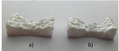
**Fig. 11.** An optical images of expanded polystyrene with (a) and without (b)  $SiO_2$  fractures incorporated into the bulk after 40 s of flame torch induced heat experiment
