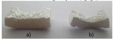
Fig. 6. An optical images of expanded polystyrene with (a) and without (b)  $SiO_2$  film after 60 s of flame torch induced heat experiment
