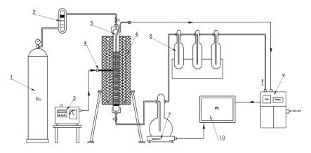
**Fig. 2.** The schematic configuration of pyrolysis experiment. 1. Nitrogen gas 2. Flowmeter 3. Temperature controller 4. Thermocouple of reactor 5. Thermocouple of sludge feed 6. Furnance 7. Balance 8. Ice bath 9. Gas analyzer 10. PC
