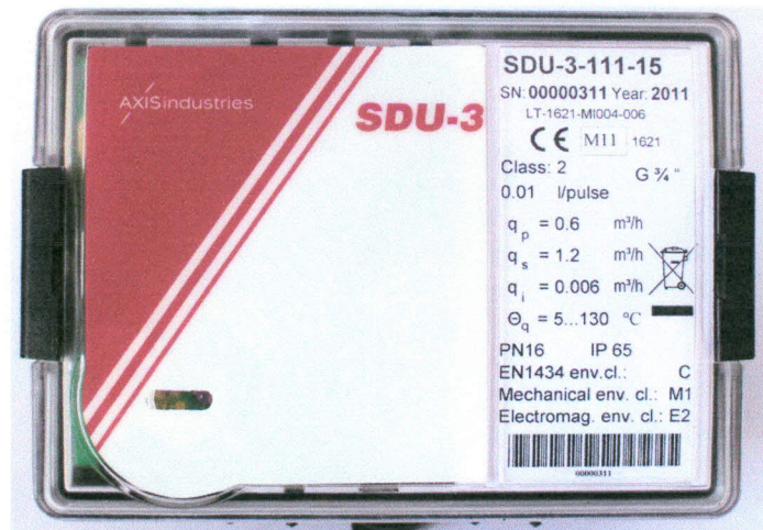
Fig.2. Electronic unit of the flow sensor
