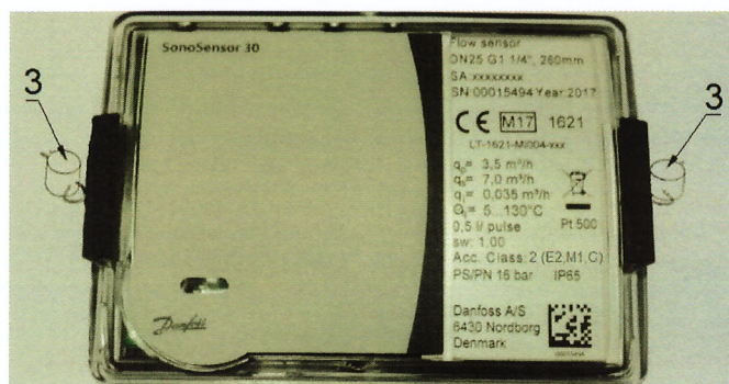
Fig.5. Sealing of the electronic unit of the flow sensor
