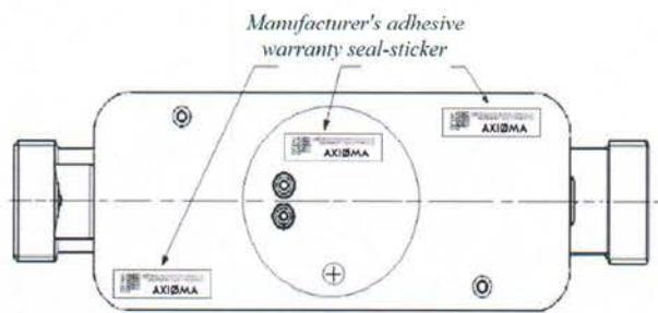
b) Sealing of flow sensor of the water meter with end connections G $\frac{3}{4}$ , G $\frac{5}{4}$ , DN25, DN32 (IP65, triangular cross-section of the meter tube)
