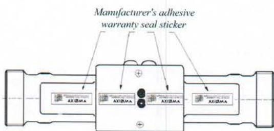
e) Sealing of flow sensor of the water meter with end connections G2; DN40; DN50; DN65; DN80; DN100 (IP65)
