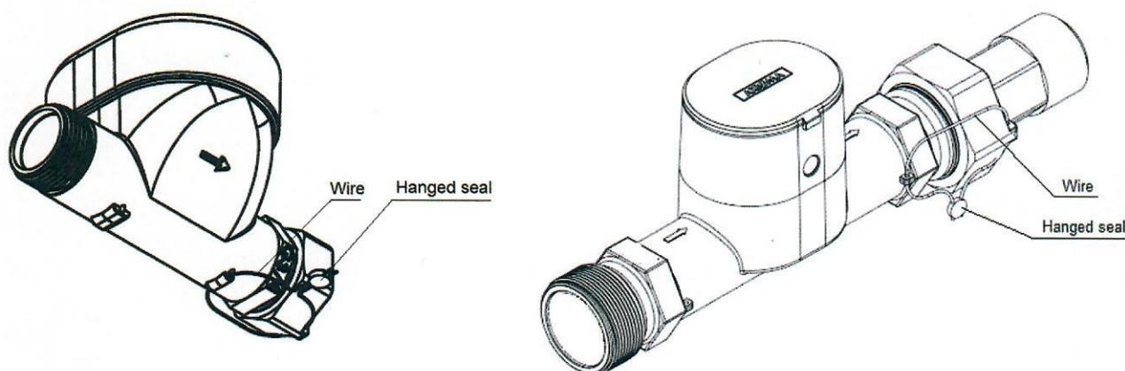
Fig.4. Sealing of the water meter QALCOSONIC W1 after installation
