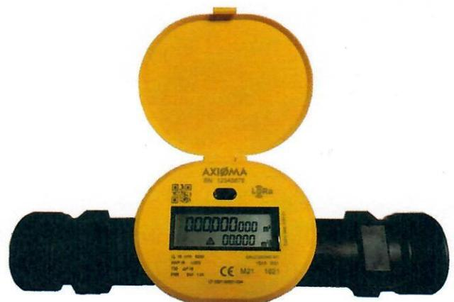
Fig. 2. Water meter QALCOSONIC W1,  $Q_3 = 6,3/10 \text{ m}^3$ , with threaded end connection G  $1\frac{1}{4}$  or G  $1\frac{1}{2}$
