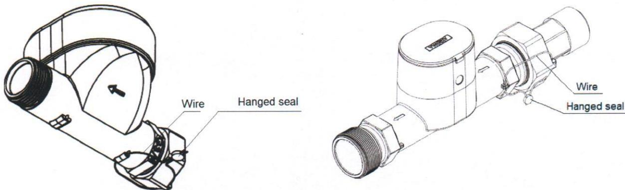
Fig. 5. Sealing of the water meter QALCOSONIC W1 after installation
