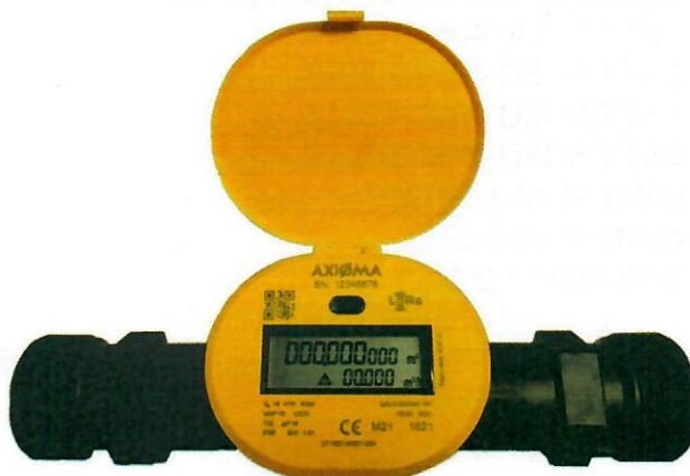
Fig. 4. Water meter QALCOSONIC W1, Q_3 = 10/16/25 \text{ m}^3 , with threaded end connection G2
