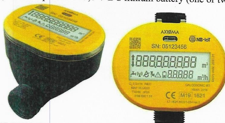
Fig.1. Water meter QALCASONIC W1, Q_3 = 1,6/2,5/4,0 \text{ m}^3/\text{h} , with threaded end connection G \frac{3}{4} or G 1 (meter design initial version)
