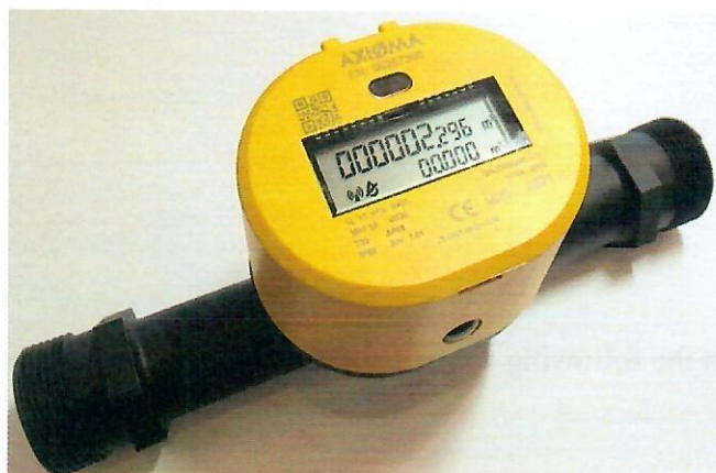
Fig. 3. Water meter QALCASONIC W1, Q_3 = 6,3/10 \text{ m}^3 , with threaded end connection G 1¼ or G 1½
