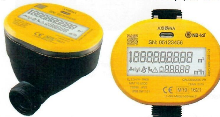
Fig.1. Water meter QALCOSONIC W1, Q_3 = 1,6/2,5/4,0 m³/h, with threaded end connection G \frac{3}{4} or G 1 (meter design initial version)
