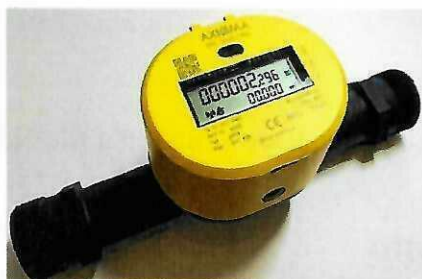
Fig. 2. Water meter QALCASONIC W1, Q_3 = 6,3/10 \text{ m}^3 , with threaded end connection G 1\frac{1}{4} or G 1\frac{1}{2}
