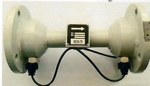
i) Measuring section of the flow sensor q_p = 25/40/60 \text{ m}^3/\text{h} with flanged end connections (DN65/DN80/DN100), steel body
