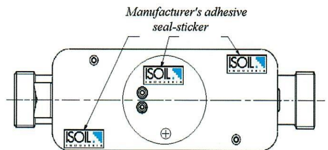
Fig. 7. Sealing of measuring section of the flow sensor q_p = 3,5/6,0 \text{ m}^3/\text{h}
