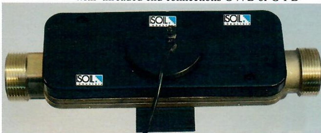
c) Measuring section of the flow sensor q_p = 3,5/6 \text{ m}^3/\text{h} with threaded end connections G 1\frac{1}{4} B
