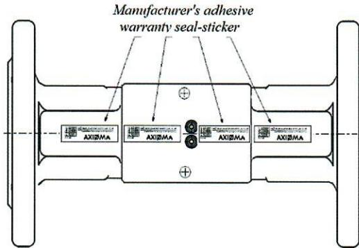
e) sealing of flow sensor  $q_p = 15/25/40/60 \text{ m}^3/\text{h}$
