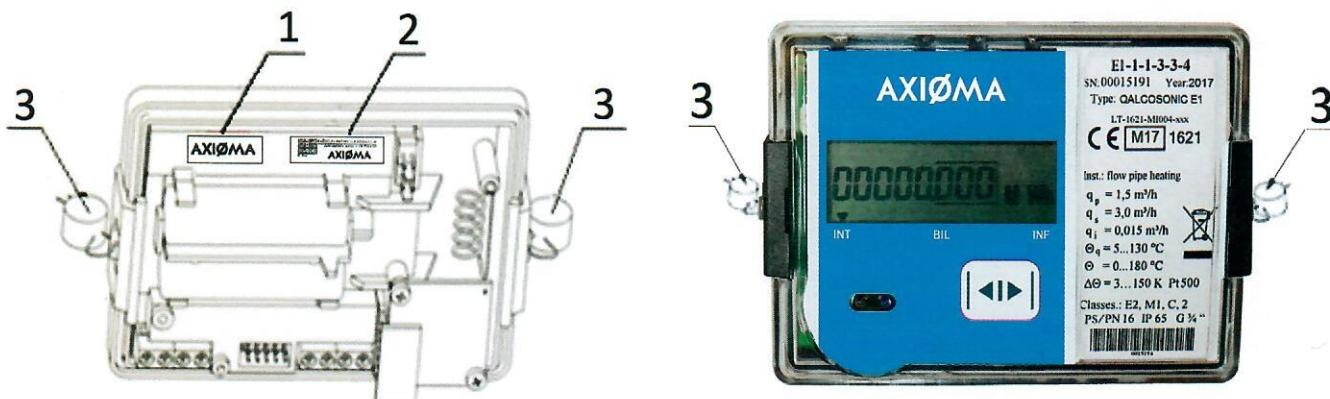
Fig.4. Sealing of the calculator of the heat meter
