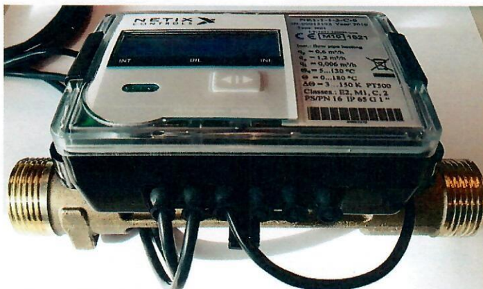
Fig.1.Heat meter NE1 (calculator and flow sensor)
