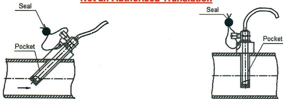
Fig. 9. Sealing of the PL type temperature probes
