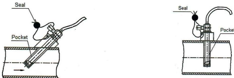
Fig. 9. Sealing of the PL type temperature probes
