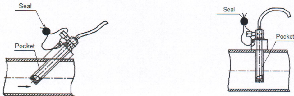
Fig. 9. Sealing of the PL type temperature probes
