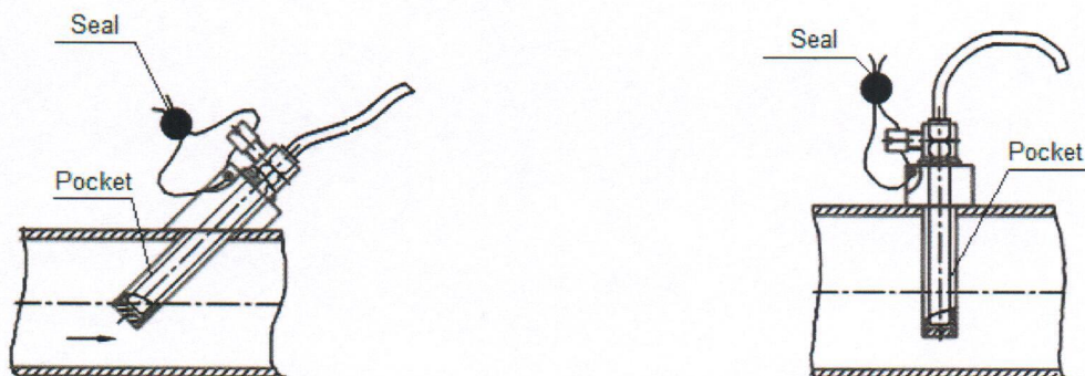
Fig. 7. Sealing of the PL type temperature probes
