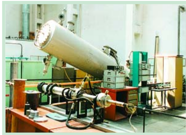
High pressure chamber for investigation of mixed convection in oblique channels
