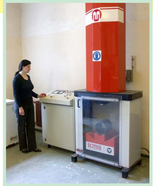
Pipe breaking facility
