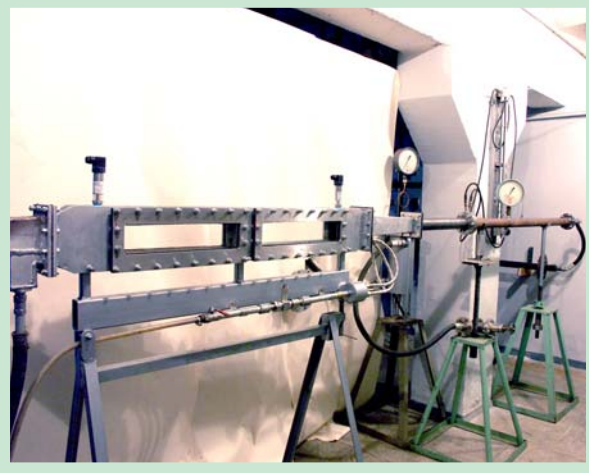
Experimental setup for two-phase flow investigation
