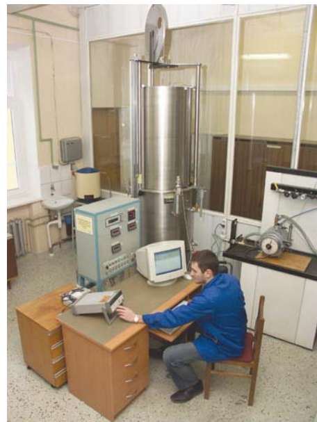
Air(gas) volume and flow rate (Part 1: 0.016-16 m 3 /h) units state standard Reference measurement instrument: bell type prover. Working volume – 0.340 m 3 . The best measurement capability of volume: \pm 0.13\%
