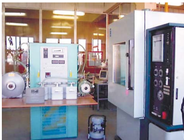
Domestic gas meters test facility with climatic chamber
