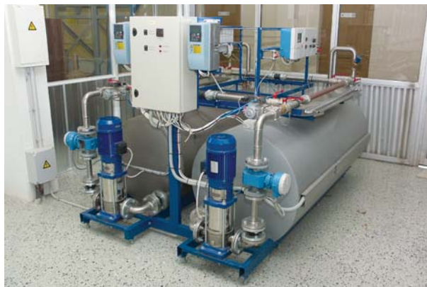
Cold and hot water meters (flow rate up to 10 m³/h) test facility
