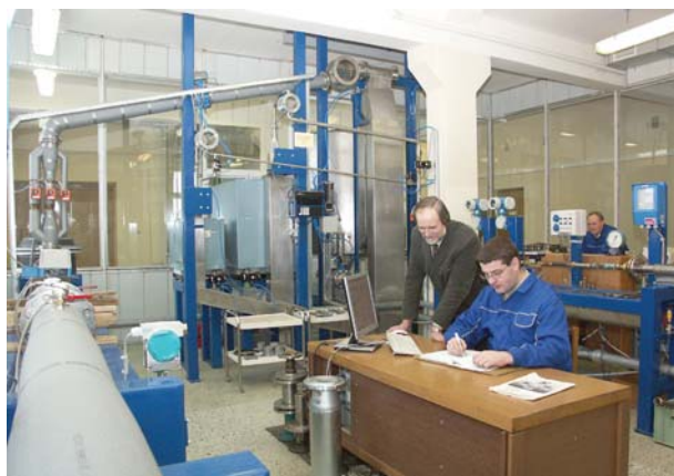
Water volume and flow rate (0.01-100 m 3 /h) units state standard Reference measurement instruments: reference scales – 60, 600 and 1500 kg. The best measurement capabilities: volume \pm 0.08\% and flow rate \pm 0.12\%
