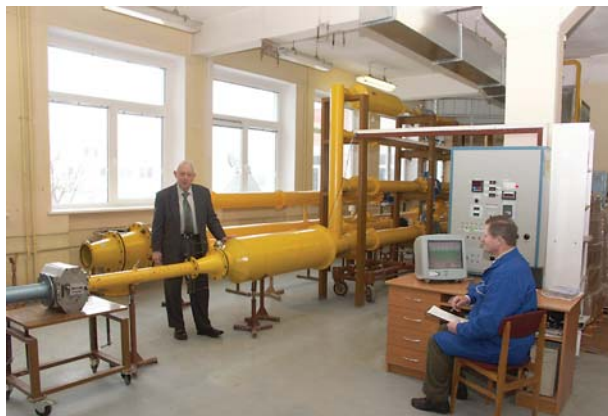
Air (gas) volume and flow rate (Part 3: 1-9750 m 3 /h) units state standard Reference measurement instruments: rotary displacement and turbine gas meters. The best measurement capabilities of volume: \pm 0.25\% , when flow rate (1-1600) m 3 /h and \pm 0.30\% , when flow rate (1600-9750) m 3 /h
