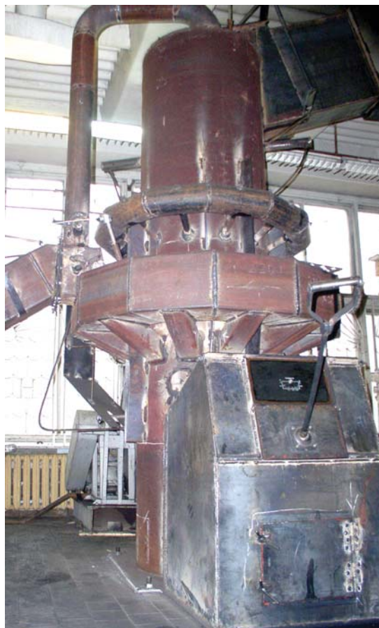
Tires gasification reactor
