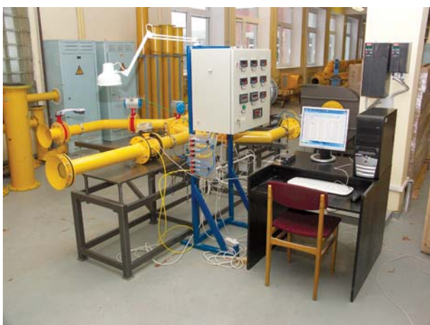
Turbine gas meters (flow rate up to 1000 m³/h) test facility
