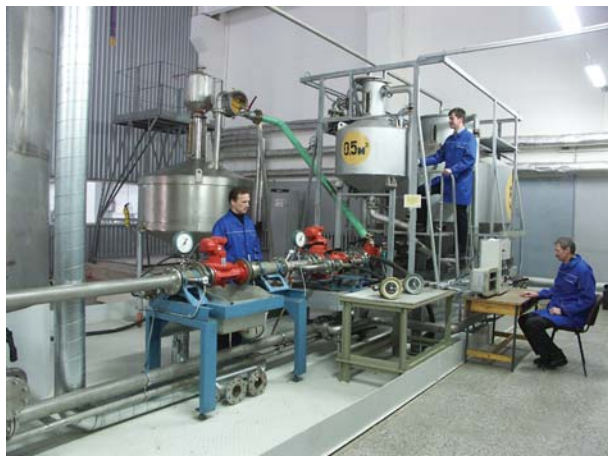
Oil products' volume and flow rate (1-120 m 3 /h) units state standard Reference measurement instruments: reference volume standards 0.5, 2 and 5 m 3 and liquid fuel meters. The best measurement capabilities: volume \pm 0.12\% and flow rate \pm 0.15\%
