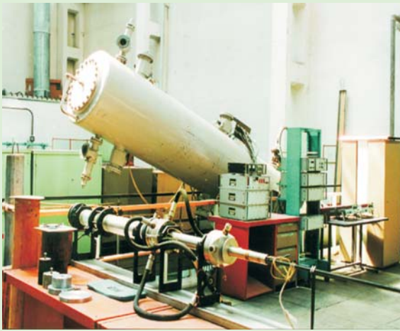
Eksperimental facility to investigate mixed convection in inclined channels
