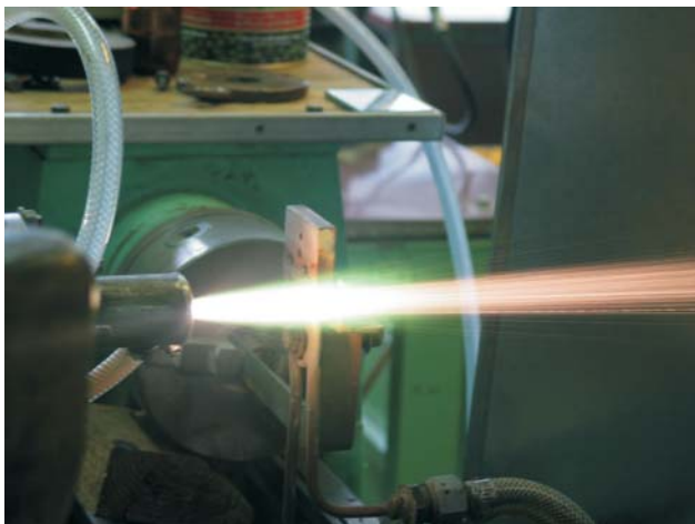
Plasma jet created by atmospheric pressure DC linear plasma generator
