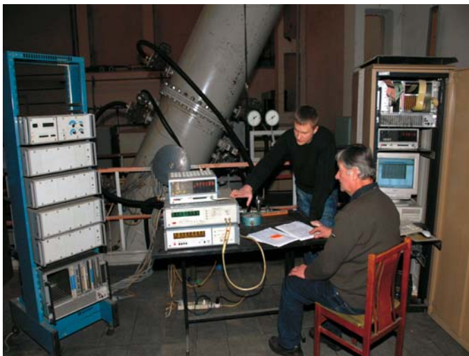
Experimental investigation of mixed convection in the inclined flat channel – Dr. J. Kolesnikovas (sitting) and PhD Candidate G. Drumstas
