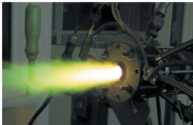
Water vapour plasma jet, flowing from 95 kW capacity plasma generator
