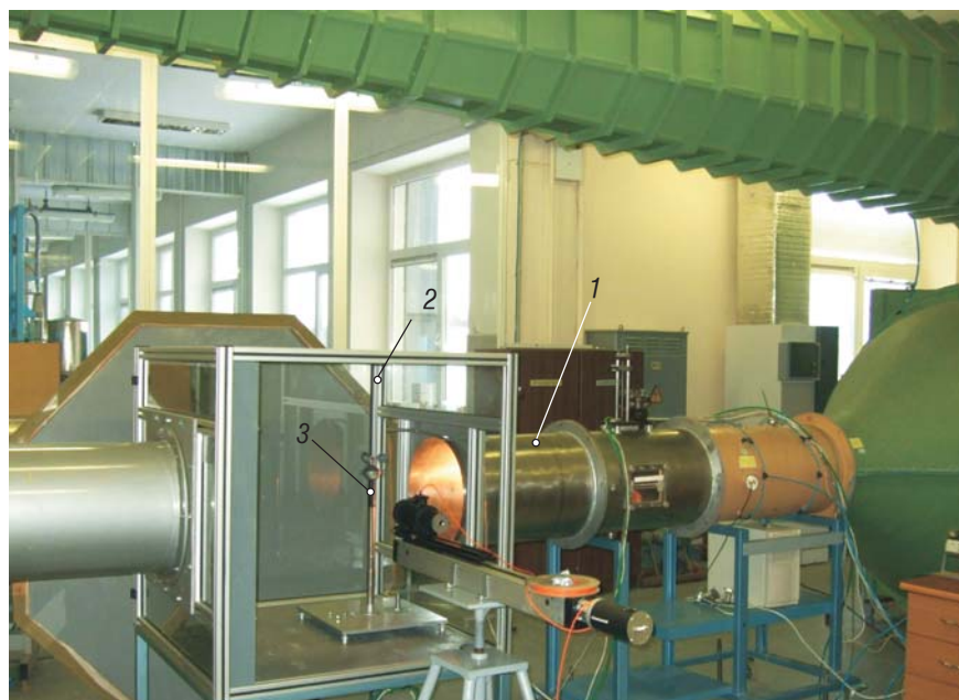
Measurement channel of aerodynamic facility, which is applied for measuring velocity in the entrance region of channel and free stream inflowing to the protective chamber, was reconstructed in 2009; 1 – measurement channel; 2 – protective chamber; 3 – object under test - wind speed meter
