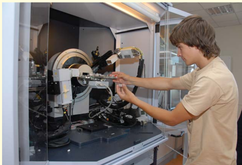
Bruker D8 Discover (Germany) X-ray diffractometer with accessories that enables carrying out the crystal structure analysis in the form of synthesized materials, thin coatings or nanopowder
