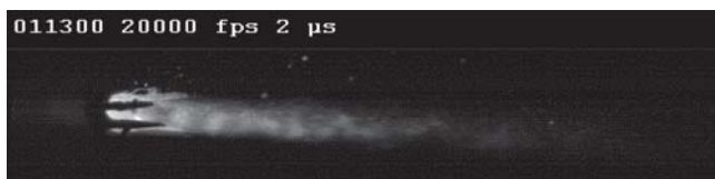
Behaviour of melted granules of zeolites in supersonic air plasma jet observed by high-speed video camera
