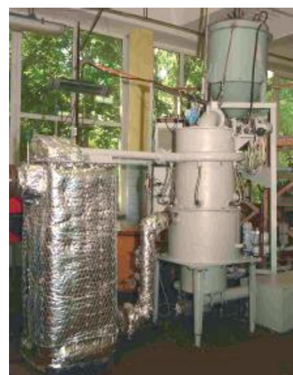
Automated experimental wood gasification reactor
