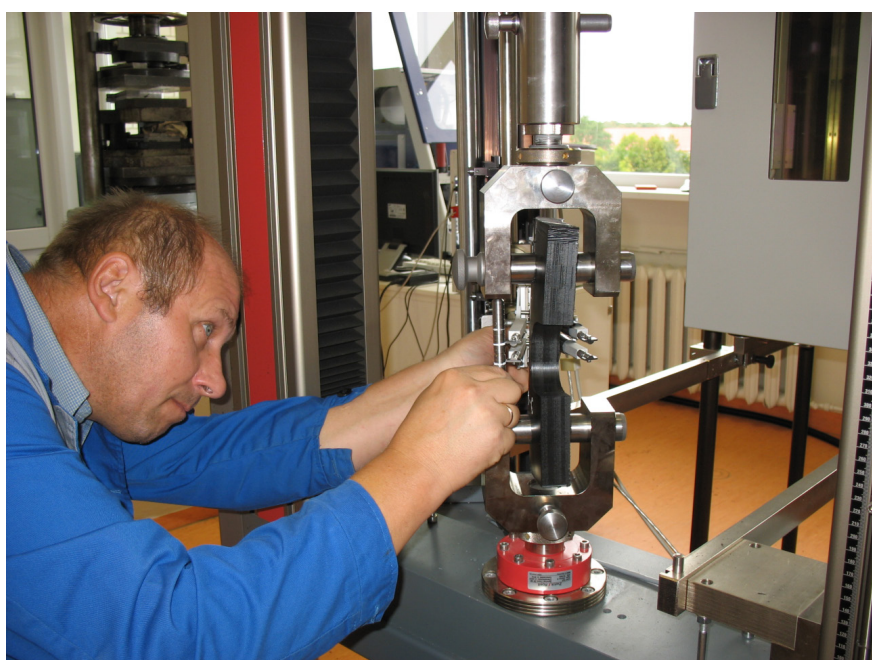
Services for customers. Testing of plastic pipes extension
