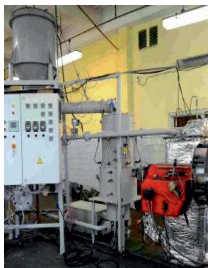
Automated experimental wood gasification reactor
