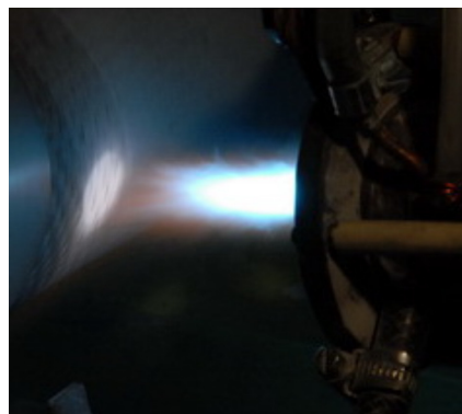
Air plasma jet discharged from constant current linear plasma generator
