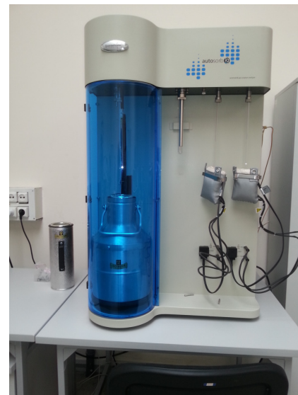
Measurement of montmorillonite specific surface area and pore size distribution; analyser of solid bodies specific surface area and pore size
