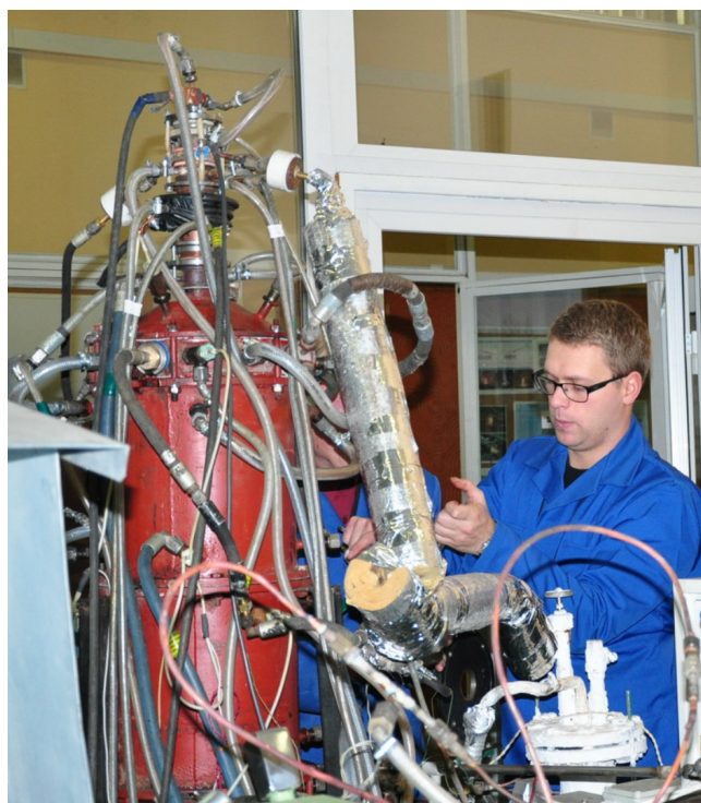
Water vapour plasma chemical reactor for the dissolving of liquid waste
