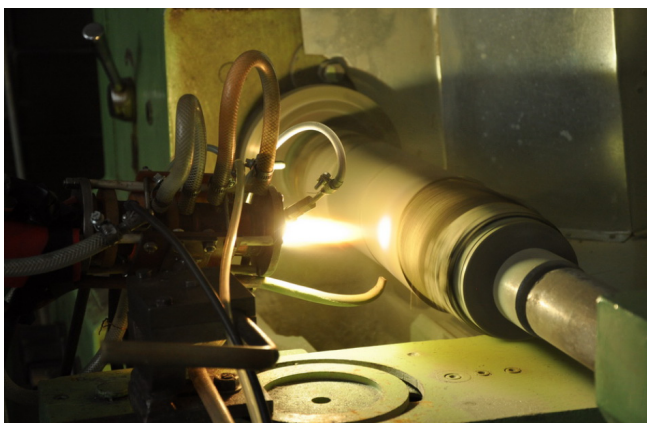
Formation of surface layers of construction materials in atmosphere pressure air plasma and examples of prepared products
