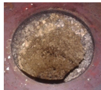
Adhesion of wood pellets in pyrolysis zone of gasification reactor
