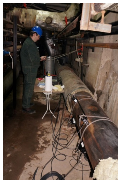
Figure 4. Junior researcher A. Bonćkus performs measurements of Marijampolė heating network in the boiler house in order to determine the reasons of imbalance
