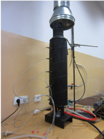
Measurement of flame emission spectra profile – spectroscope is connected with optical fibers
