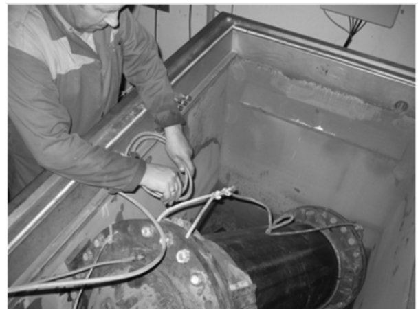
Services to customers. Testing of plastic pipe (determination of resistance to internal pressure)
