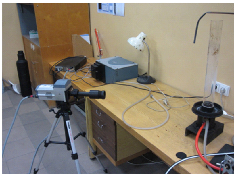
Laboratory burner and camera for spectroscopic analysis of flame
