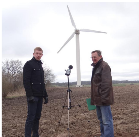
Noise measurements conducted nearby 250 kW capacity WPP
