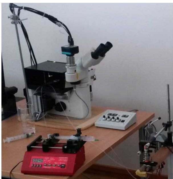
Fig. 2. Device for investigation of flows in micro-channels
