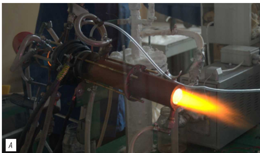
Water vapour plasma torches for the organic waste treatment. A – the conversion of hydrocarbon gases, B – the conversion of liquid and solid wastes
