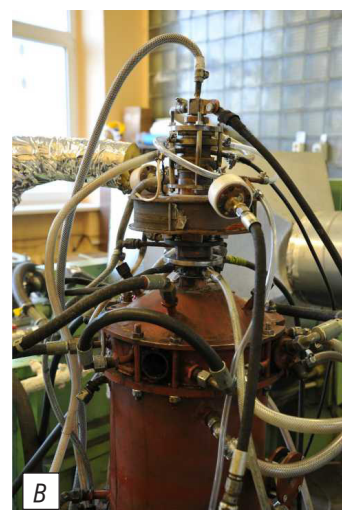
Water vapour plasma torches for the organic waste treatment. A – the conversion of hydrocarbon gases, B – the conversion of liquid and solid wastes
