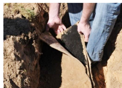
Collection of geomembrane sample buried near Maišiagala repository
