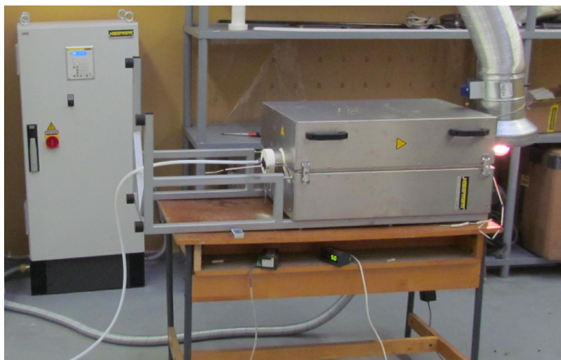
Electrical tube furnace Nabertherm RS 80/500/13 with temperature control unit
