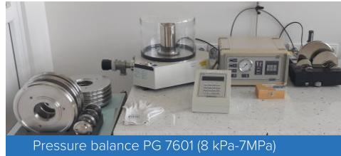
Pressure balance PG 7601 (8 kPa-7MPa)
