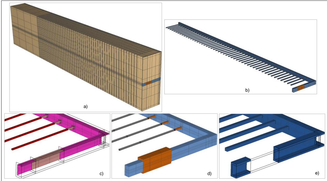
**Fig. 2.6.** Computational grid of the repository module coloured by material type: a) full modelling domain; b) system of the tunnels and the EDZ; c) interfaces; d) engineered barriers; e) the EDZ
