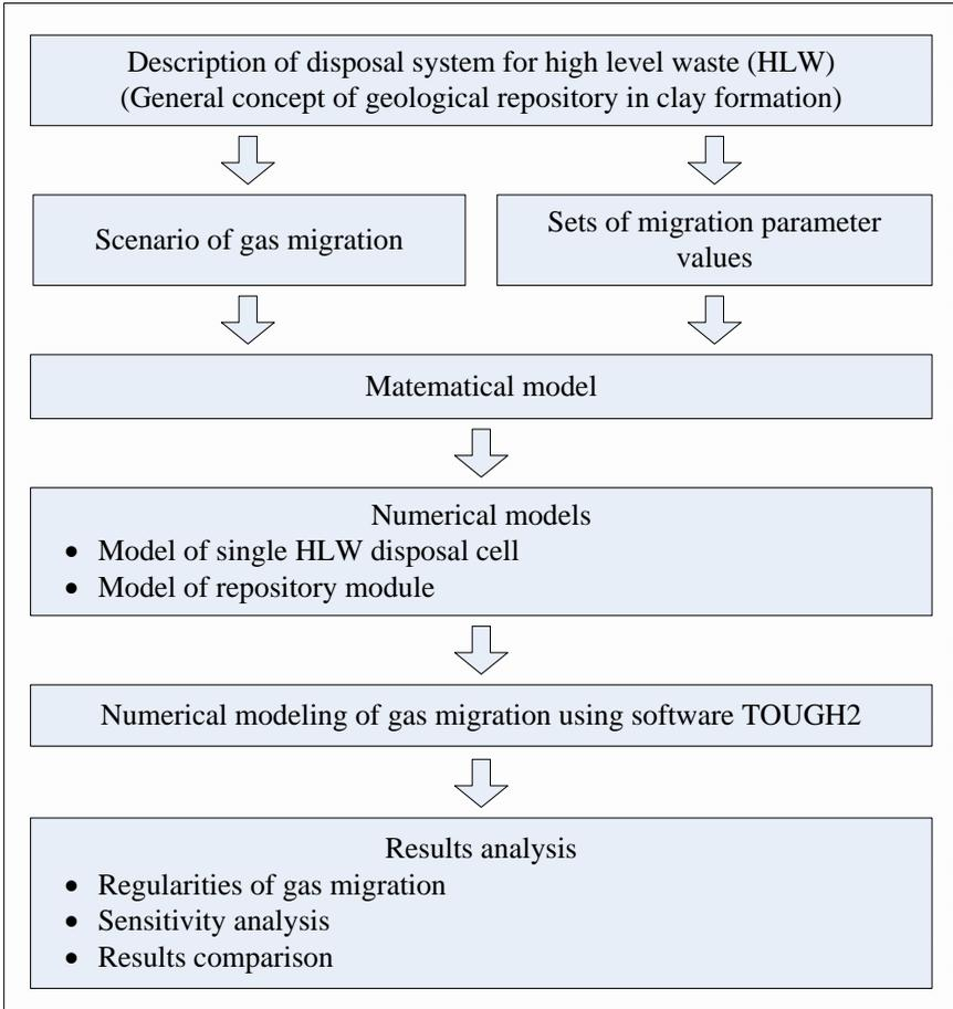
**Fig. 2.1.** Methodology for the analysis of gas migration in the geological repository
