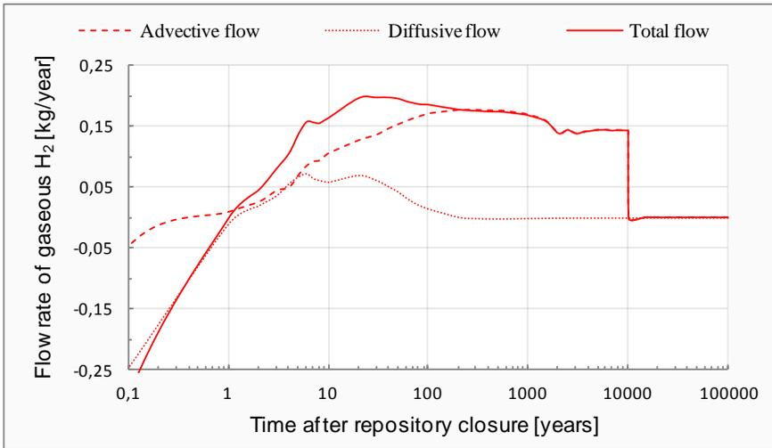
**Fig. 3.4.** Evolution of gaseous H<sub>2</sub> flux towards the access drift
