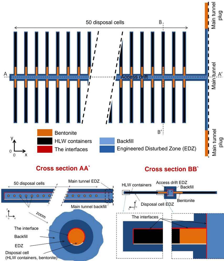
**Fig. 2.3.** Geological repository module [3]
