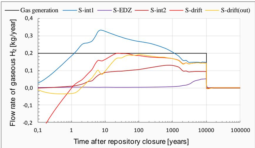
**Fig. 3.3.** Evolution of gaseous  $H_2$  flux through different surfaces
