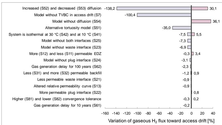
**Fig. 3.6.** Comparison of gaseous  $H_2$  flux towards the access drift for all analysed cases
