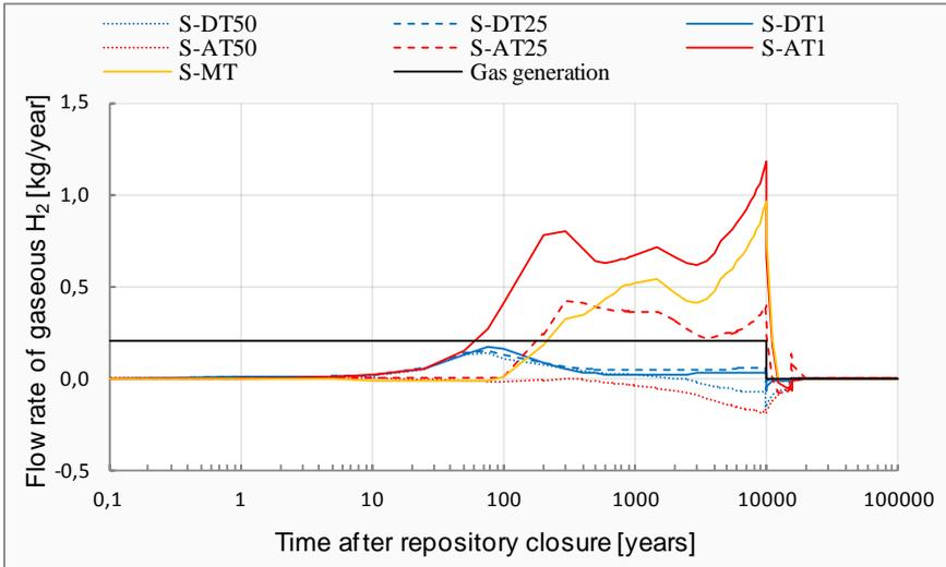
**Fig. 3.10.** Evolution of gaseous H<sub>2</sub> flux through different surfaces
