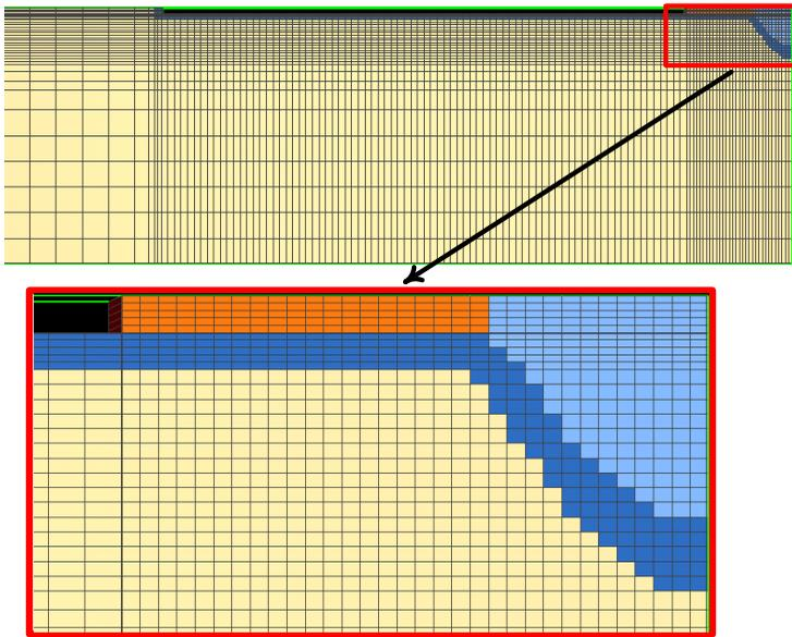
**Fig. 2.5.** Computational grid of a disposal cell model
