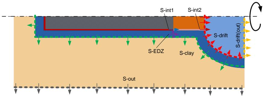
**Fig. 2.8.** Observation surfaces and directions of fluid fluxes in a single disposal cell model
