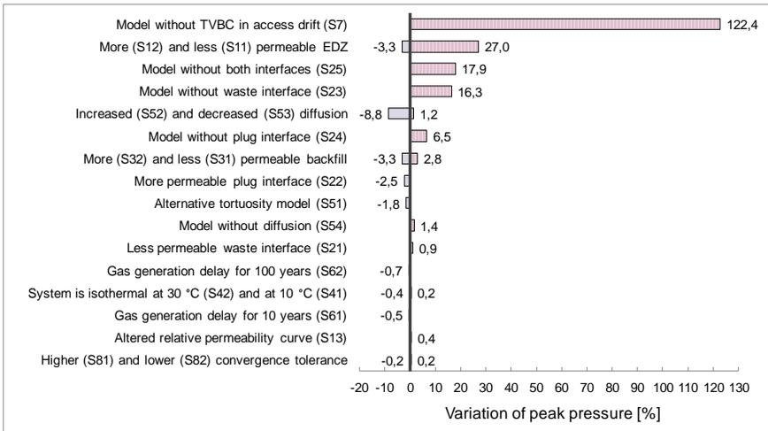
**Fig. 3.5.** Comparison of peak pressure in the system for all analysed cases
