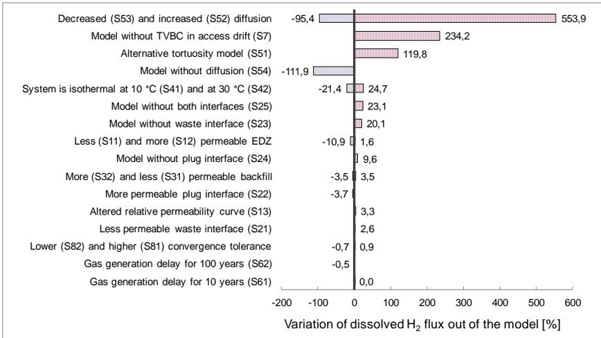
**Fig. 3.7.** Comparison of dissolved H<sub>2</sub> flux out of the model for all analysed cases
