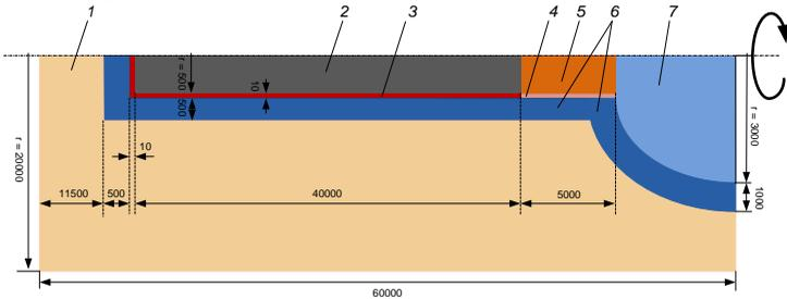
**Fig. 2.4.** Model of a single disposal cell: 1 – undisturbed clay formation; 2 – HLW containers; 3 – waste interface; 4 – bentonite plug interface; 5 – bentonite plug; 6 – engineered disturbed zone (EDZ); 7 – access drift
