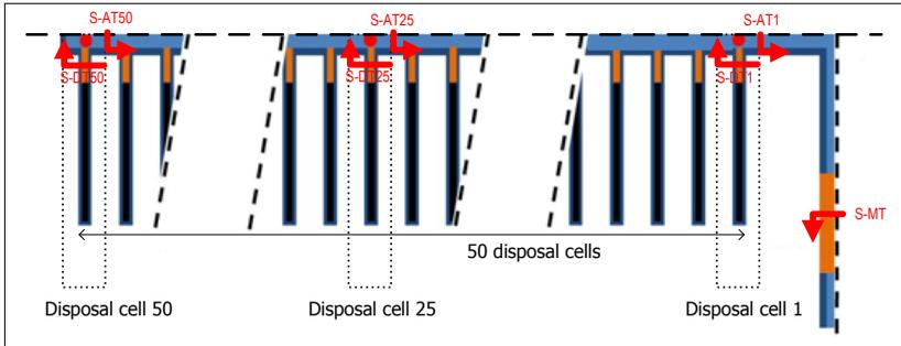
**Fig. 2.10.** Observation surfaces and directions of fluid fluxes in the repository module model
