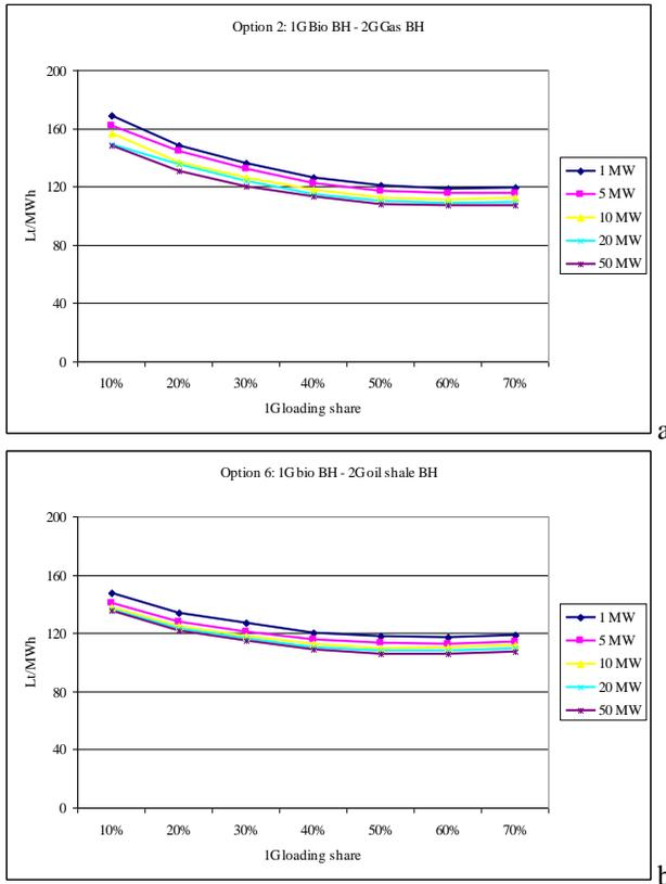
**Fig. 21.** Heat generation costs for various boiler-house capacities, when 1G is biofuel boiler and 2G is a)– gas boiler; and b) shale oil boiler
