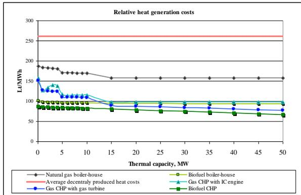
**Fig. 14.** Relative heat generation costs for 5 selected heat generation technologies in boiler-houses and CHP plants comparing to decentralized heat generation costs
