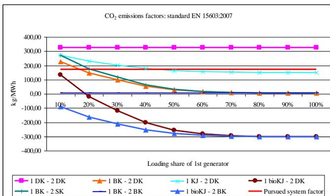
**Fig. 19.** CO<sub>2</sub> emission factors vs. change of maximal capacity share of 1G using standard fuel coefficients under EN 15603:2007
