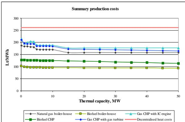
**Fig. 13.** Summary production costs for 5 selected heat generation technologies in boiler-houses and CHP plants comparing to decentralized heat generation costs
