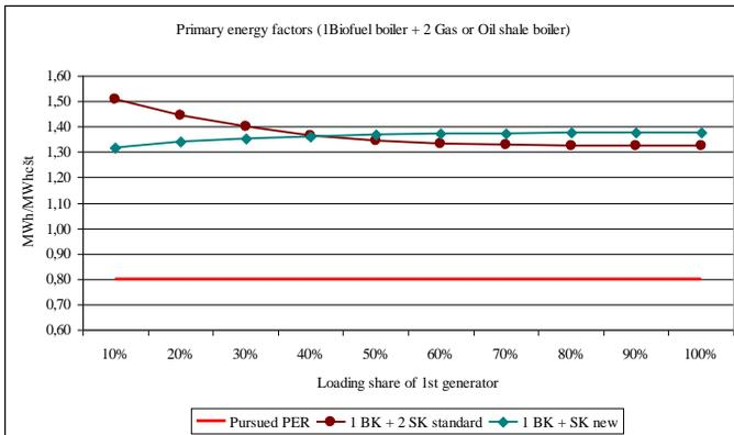
**Fig. 16.** *PER* vs. change of maximal capacity share of 1G using standard and new fuel coefficients, when 1G – biofuel boiler and 2G is natural gas or oil shale boiler
