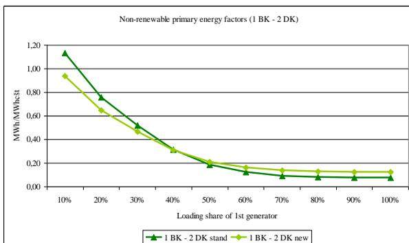
**Fig. 18.** *NPER* vs. change of maximal capacity share of 1G using standard and new fuel coefficients, when 1G is biofuel boiler, and 2G is natural gas or oil shale boiler
