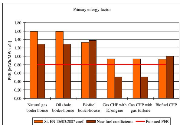
**Fig 11.** Primary energy factors for 6 selected heat generation technologies at standard and newly prepared fuel primary energy coefficient and pursued  $PER$
