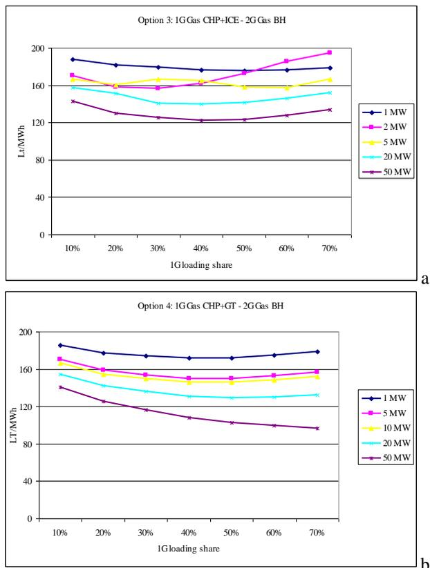
**Fig. 22.** Heat generation costs for various boiler-house capacities, when: a) 1G is natural gas CHP with internal combustion engine, and 2G – natural gas boiler; b) 1G natural gas CHP with gas turbine, and 2G is natural gas boiler
