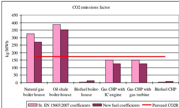
**Fig. 12.** CO<sub>2</sub> emissions factors 6 selected heat generation technologies at standard and newly prepared fuel CO<sub>2</sub> coefficients and pursued CO<sub>2</sub>R
