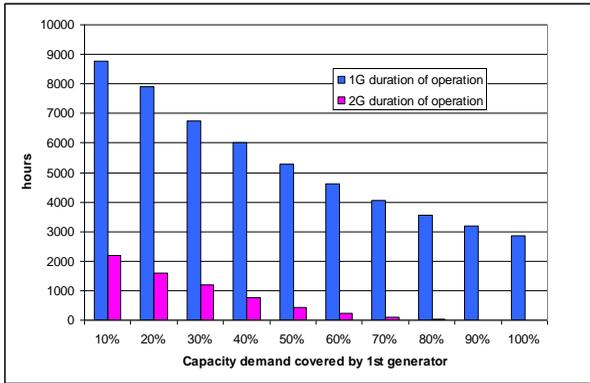
**Fig. 15.** Distribution of heat generation duration between 1G and 2G at full loading vs. change of maximal capacity share of 1G
