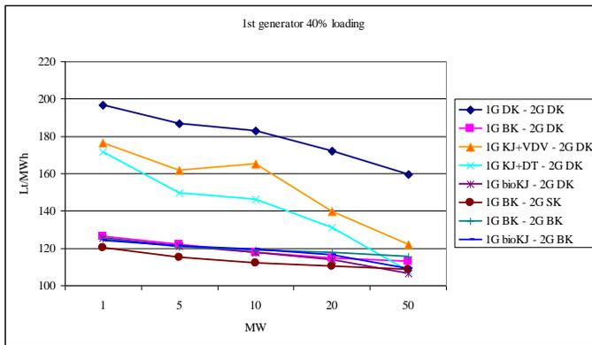
**Fig. 24.** Comparison of heat generation costs for various technologies when 1 generator covers 40% of heat capacity demand
