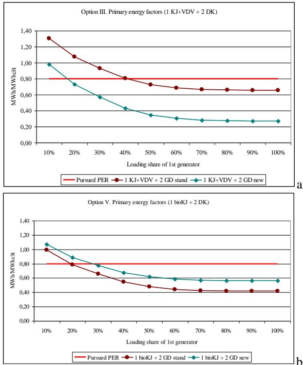
**Fig. 17.** PER vs. change of maximal capacity share of 1G using standard and new fuel coefficients, when 2G – natural gas boiler; and 1G is a - CHP unit with internal combustion engine or gas turbine and b - biofuel CHP unit
