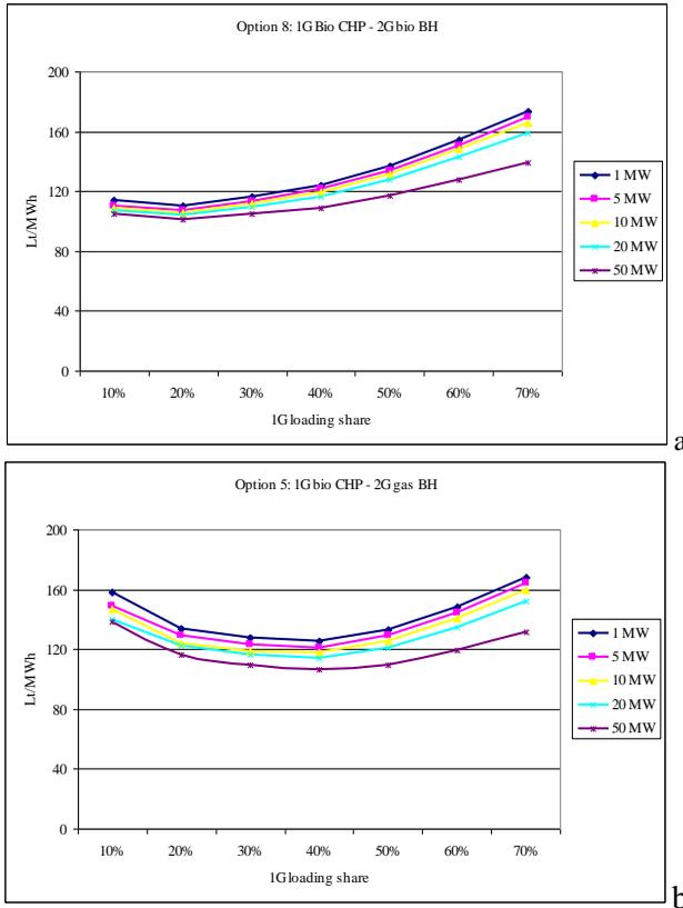
**Fig. 23.** Heat generation costs for various boiler-house capacities, when: a) 1G is biofuel CHP and 2G is biofuel boiler; and b) 1G is biofuel CHO and 2G is natural gas boiler.
