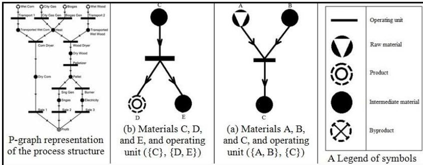
**Figure 3.** Principle of PNS structure using P-graph method
