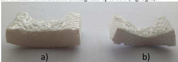
**Fig. 6.** An optical images of expanded polystyrene with (a) and without (b) SiO<sub>2</sub> film after 60 s of flame torch induced heat experiment
