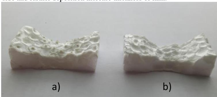
**Fig. 11.** An optical images of expanded polystyrene with (a) and without (b) SiO<sub>2</sub> fractures incorporated into the bulk after 40 s of flame torch induced heat experiment
