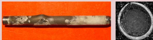
(MTA EK burst test sample available in the database)
