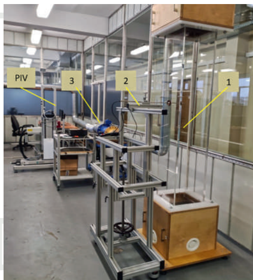
1 – vertical channel with particle movement visualization system - PIV; 2 – control device of test object (TO); 3 – section for air flow meter; 4 – section for solid particle (PM) injection; 5 – bipolar PM agglomerator; 6 – fan
