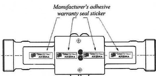
e) Sealing of flow sensor of the water meter with end connections G2; DN40; DN50; DN65; DN80; DN100 (IP65)
